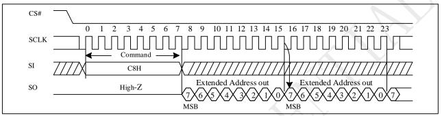
Figure 9-9a Read Extended Address Register Sequence (QPI)
