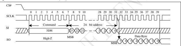
Figure 9-61 Read Block Lock Status (SPI)
