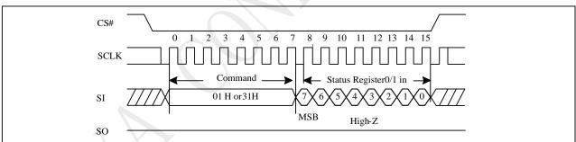
Figure 9-7 Write Status Register (WRSR) Sequence (SPI)
