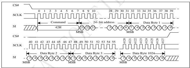
Figure 9-47a Program Security Registers (PRSCUR) Sequence (QPI)
