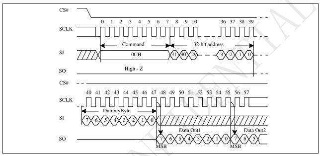
Figure 9-17 Fast Read with 4-Byte Address Sequence (SPI)
