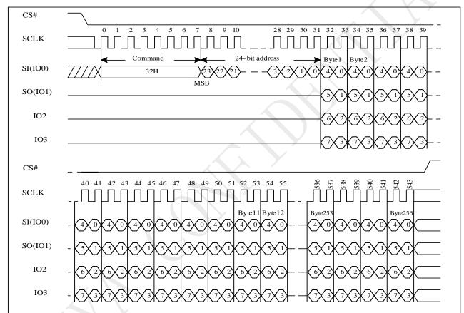
Figure 9-42 Quad Page Program (QPP) Sequence (SPI)
