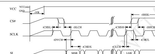
Figure 5-8 AC Timing at Device Power-Up
