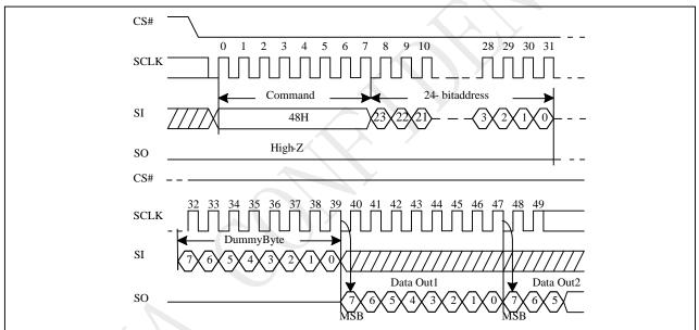
Figure 9-48a Read Security Registers (RDSCUR) Sequence (QPI)
