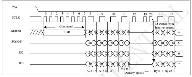
Figure 9-27 DTR 4IO Read Mode Sequence (SPI, M5-4 ≠ (1,0))
