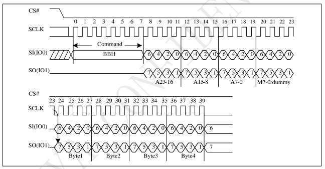
Figure 9-20 2IO Read Sequence (SPI, M5-4 ≠ (1,0))
